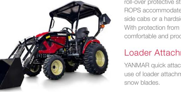
The Model SA425DHF offers an optional four-post roll-over protective structure (ROPS). The 4-post ROPS accommodates installation of optional soft-side cabs or a hardside cab with optional heater. With protection from the cold or rain, you'll be more comfortable and productive.
